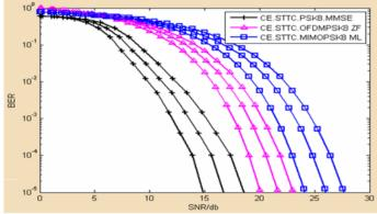
Fig.5. Channel estimation in the STTC for OFDM-MIMO with fourth Generation wireless system with 8-PSK
