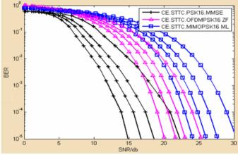
Fig.6. Channel estimation in the STTC for OFDM-MIMO with fourth Generation wireless system with 16-PSK
